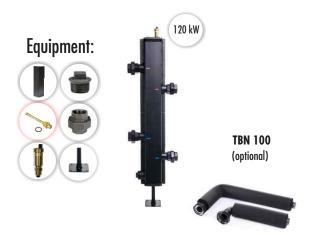
Hydraulic separator CPN 100 DN 40 is made of steel. The factory is equipped with insulation, and the upper side with two connections for the temperature sensor and a vent (coupler 1/2 "M), and the lower side of the drain connection (coupler 2" F). In the set they are automatic air vent 3/8" with check valve 1/2", immersion sleeve for temperature sensor  $\frac{1}{2}$ ", four cast-iron fittings 1  $\frac{1}{2}$ " and mounting feet.
